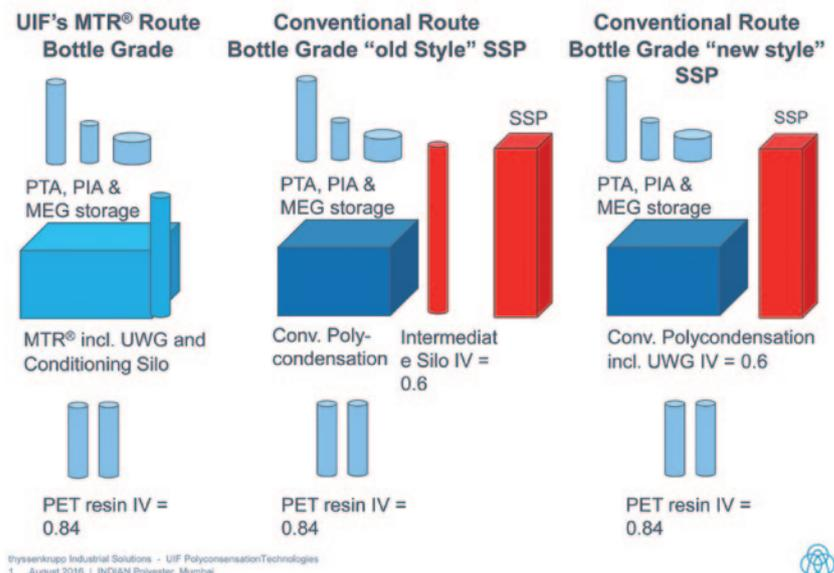
Fig. 1: Process block diagram of the three competing concepts for production of bottle grade PET resin
