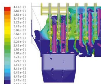
CFD simulation of a detail at the DISCAGE® for PBT
