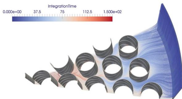
CFD simulation of a detail at the ESPREE® reactor for PET
